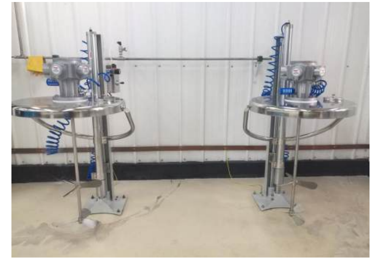
200L High power pneumatic lifting mixer
