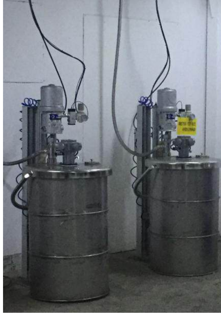
200L High power pneumatic lifting mixer
